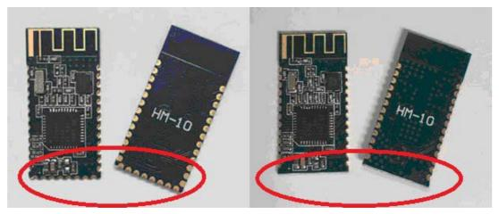
Left is HM-10S, it has 34 Pads. Right is HM-10C and it only have 26 Pads HM-10C is cheaper than HM-10S.
